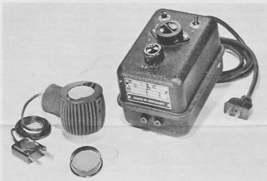
Modern microscopes are almost invariably used with artificial light sources; the most simple of which is a 15 Watt 110 Volt lamp, mounted on a pin which fits into the microscope base under the condenser. This lamp is satisfactory for most observations through a monocular tube, even under highest magnifications (1250 x).
