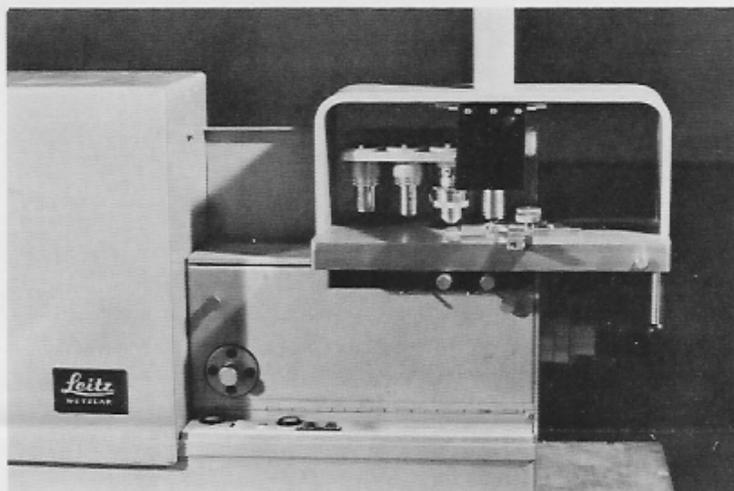
Microprojection is one of the oldest teaching aids in medical study and diagnosis. Recent developments in high-power Xenon lamps have permitted the design of projectors without troublesome, noisy carbon arc lamps. The well-known Leitz Microprojector XIc has been re-designed and is now equipped with a Xenon 450 Watt lamp which facilitates group demonstrations to an extent never before possible.
