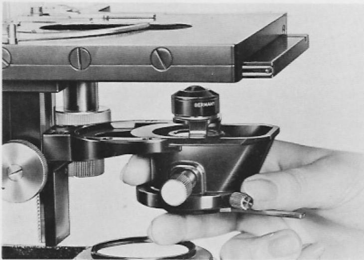
The upper condenser elements are interchangeable, so that only one basic condenser need be furnished. The operation of the new condensers is very similar to the "Berek" type. The aperture diaphragm is on the condenser proper, but the field stop is in the base of the microscope stand operated by a knurl. Condenser #602 fits into the dovetail fork of the substage and has its own centering device.
