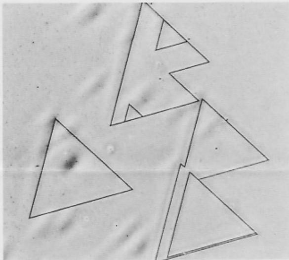
Stacking faults on semiconductor wafer surfaces have extremely low relief. Reflected light phase contrast proves in some cases to be an ideal method of observation due to this method's high sensitivity to detection of minute optic path differences.
