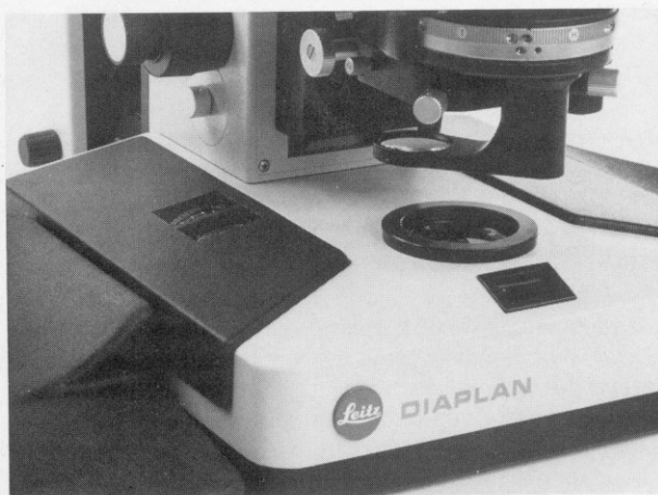
Fig. 3: Control of the aperture and field diaphragm in the base of the microscope.
