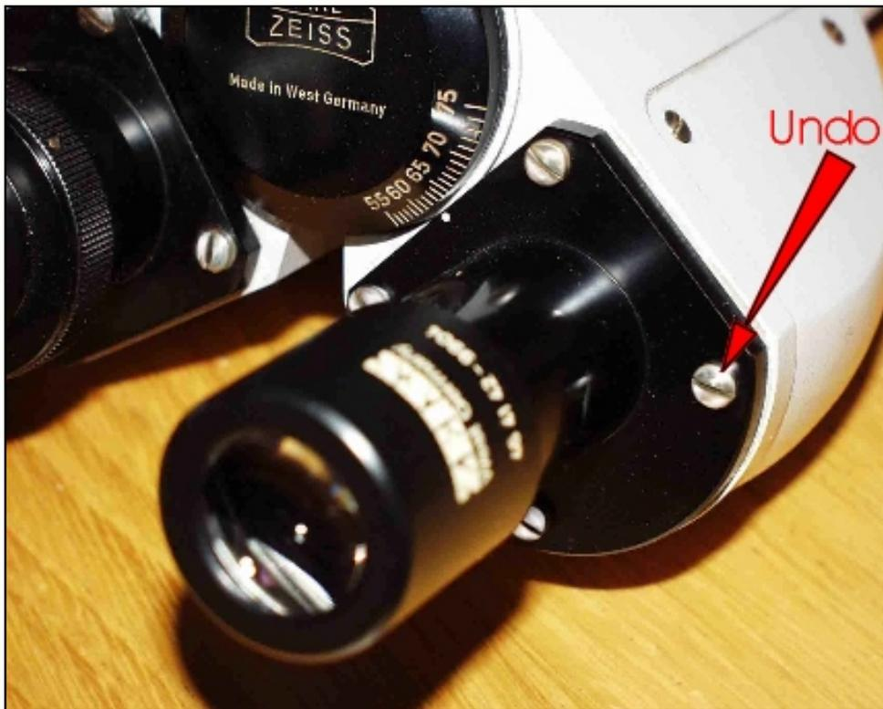
If you are going to attempt dismantling any part of a microscope you must be prepared. Only the best quality tools will do. Screwdrivers must be the correct width and thickness for each screw, cheap tools will be a disaster (mainly to the finish and screw heads). Working on a binocular head requires a scrupulously clean area and great care not to touch optics. If you decide to adjust your Wild heads read through the instructions first, it is basically easy but needs care and a lot of patience.
