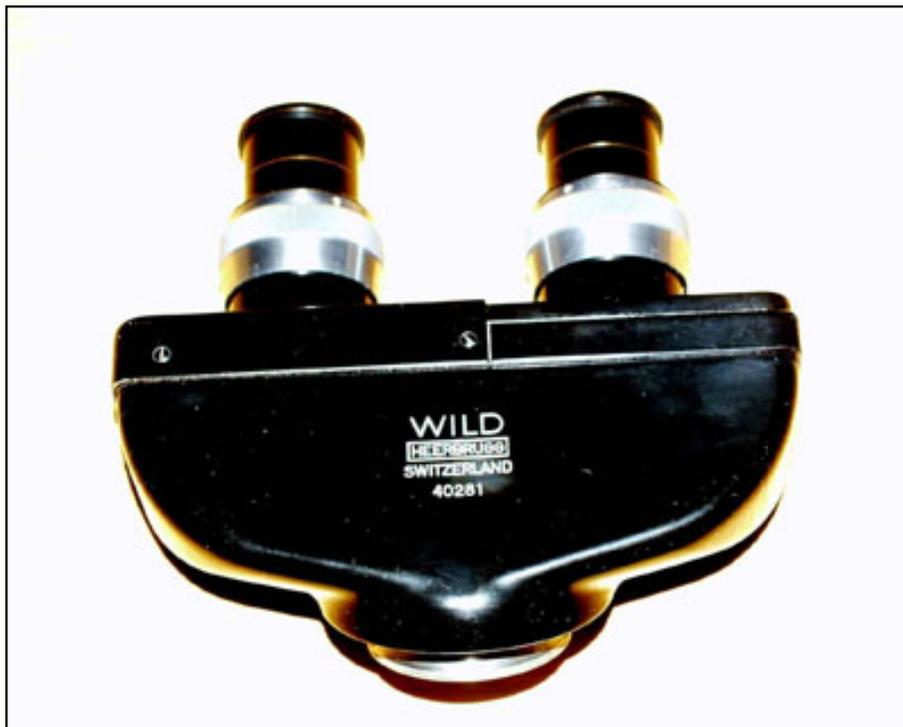
On inspecting the Wild heads I found there are two main types. One standard type with left eye individual focus, and one type with two focussing eye tubes (for
