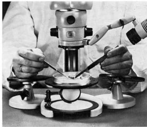
9 Hand rests, 47 52 68, facilitate dissecting work. They can be vertically adjusted as well as tilted and turned by means of ball-and-socket joints.
