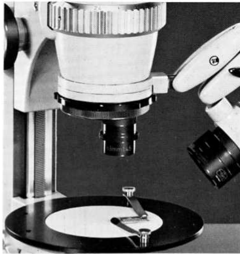
26 63 mm LUMINAR attached in place of the main objective
