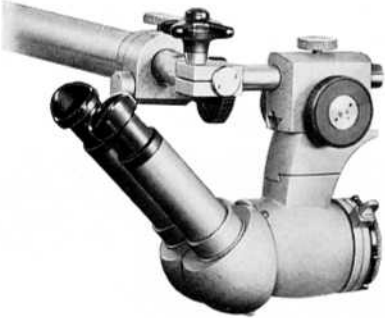
20 For observing vertical surfaces, the stereomicroscope is set up in this manner
