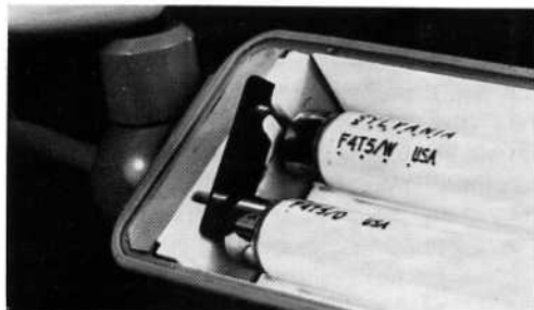
8 Diffuse-light illuminator: After inserting the fluorescent tubes, replace the plastic clip.
