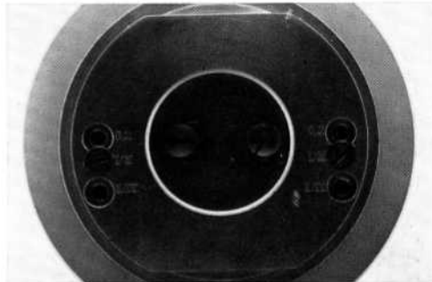
14 Underside of trans-illuminator: stop screws, here set for Stereomicroscope I or III
