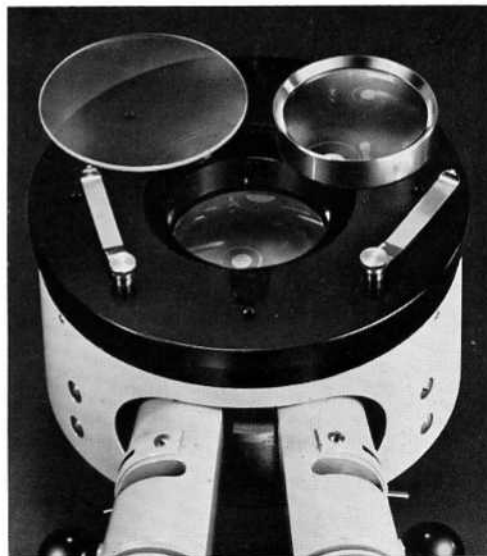
15 The auxiliary lens is exchanged only if the equipment is to be used in conjunction with another type of stereomicroscope (see table on left).
