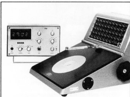
Particle Size Analyzer TGZ 3A for Automatic Data Analysis Measures and counts particles directly from electron micrograph or photomicrograph. Of great value in air pollution studies. Provision for on-line or off-line computer analysis. Shown here is the automatic model.
